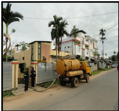
Mechanical collection of septage
